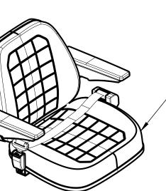
Supplier's logo is not allowed to be visible. Serial number must be available for tracing. Seat cushion heating and seat belt included as standard features in seat delivery.
